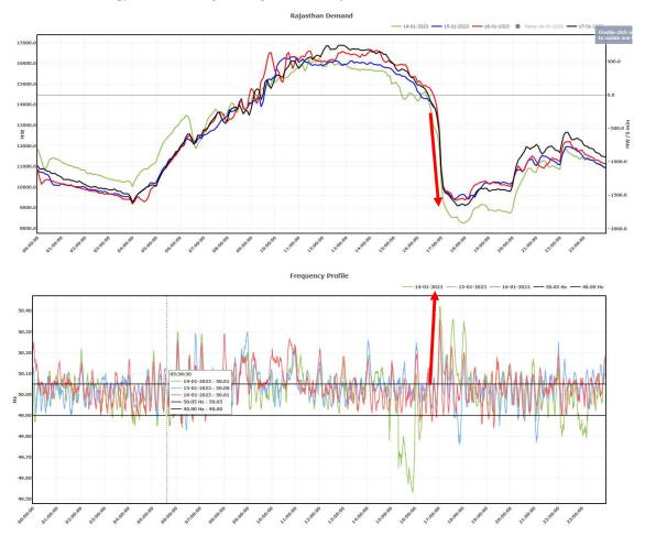
Such action by Rajasthan is leading to high voltage and high frequency at the time of sudden disconnection of load and has also lead to tripping of important lines on overvoltage. This needs to be immediately stopped by Rajasthan considering system security and staggering of load connection/ disconnection needs to be implemented at the earliest.
