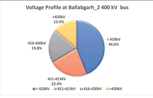
From above, it may be seen that 400kV Ballabgarh S/s voltage remained >415 kV for about 34% time. Considering above and the high voltage prevailing in NR grid, it is recommended to replace 420 kV 80MVAr bus reactor at Ballabgarh with 420 kV 125 MVAr bus reactor.
