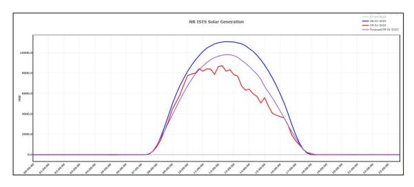
A.13.5 In the view of above the frequency even touched to 49.41Hz between 14:45 Hrs to 15:00 Hrs. Further continuously low grid frequency was observed from 11:00 Hrs to 16:00 Hrs during under injection of NR ISTS connected RE plants.
