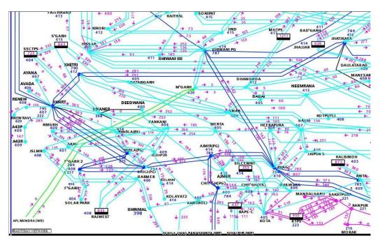
It can be seen that grid voltages are well within limits in Western Rajasthan at both intrastate as well as interstate substations.
